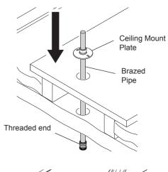
Centralise the brass pipe in the hole then screw the ceiling mount plate to the wooden support.
