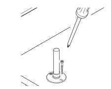
5. Offer the Ceiling-Fed Arm to the brass pipe and determine the showering height required. Push or pull the brass pipe using a twisting motion to adjust the height. Check the height is correct and use a 15 mm pipe cutter to cut the pipe to the desired length. **Note!** Cut the brass pipe at least 30 mm above the ceiling mount plate to allow room to fit the olive, nut and elbow.
